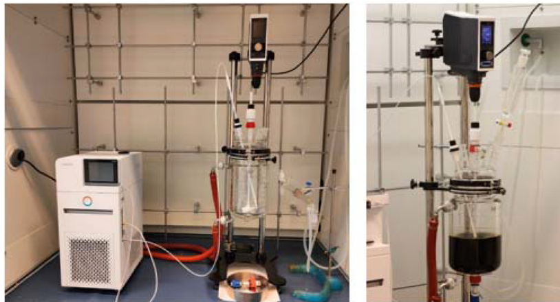
Chart 1 The 5 L stirred reactor used for the upscaled synthesis of lignin LPO.
