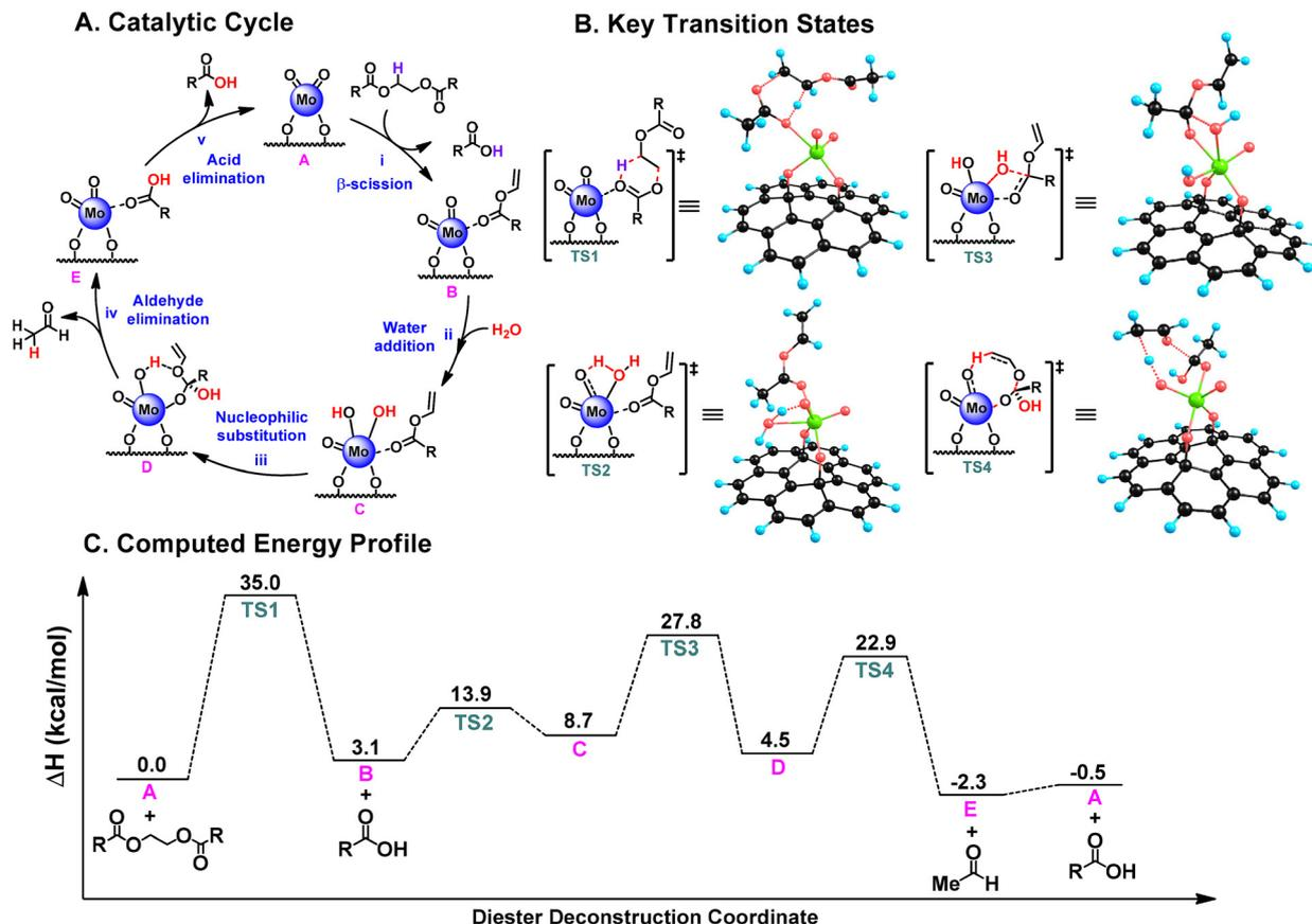
**Fig. 3** DFT analysis of diester deconstruction catalyzed by AC/MoO<sub>2</sub>. (A) Computed catalytic cycle. (B) Key transition states. Green = molybdenum, black = carbon, red = oxygen, light blue = hydrogen (C) computed enthalpy profile in kcal mol<sup>-1</sup>. R = Me in computational studies.
