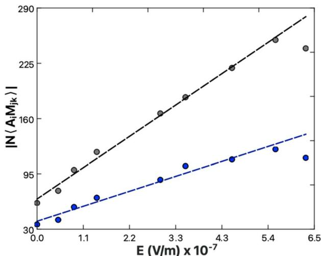
Fig. 7  $3200\text{ cm}^{-1}$  (black) and  $3400\text{ cm}^{-1}$  (blue) peak transition probabilities from spectral fits of Ca-exposed DPPS (Fig. 5B) plotted as a function of the electric field strength one Debye length away from the lipid surface (Table 1). The determined slopes, representing the relative  $\chi^{(3)}$ , are  $3.4 \pm 0.1 \times 10^6\text{ m V}^{-1}$  for the ice-like  $3200\text{ cm}^{-1}$  and  $1.6 \pm 0.1 \times 10^6$  for the water-like  $3400\text{ cm}^{-1}$ .
