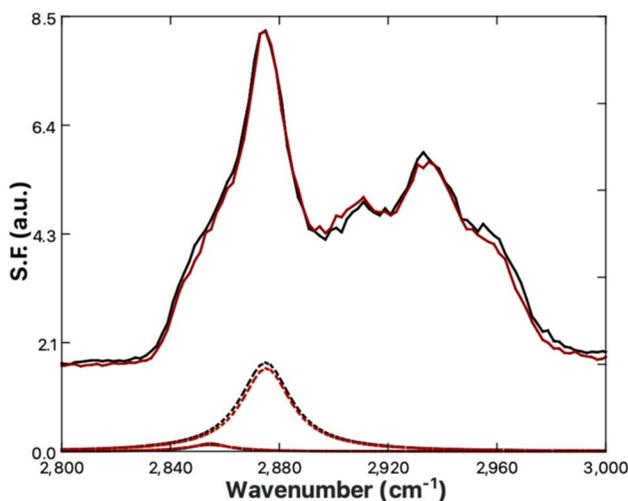
Fig. 9 SFVS spectra of DPPS in  $\text{D}_2\text{O}$  with  $100\text{ mM KCl}$  (black) or  $40\text{ mM CaCl}_2$  (red). The offset curves (dashed lines) are the spectral fits of the  $\text{CH}_2 \nu_s$  and  $\text{CH}_3 \nu_s$  peaks at  $2850\text{ cm}^{-1}$  and  $2875\text{ cm}^{-1}$  respectively, obtained using eqn (4). All solutions were buffered with Tris at  $\text{pH} = 7.4$  with a total ionic strength of  $133.4\text{ mM}$ . Spectra were recorded at  $21\text{ }^\circ\text{C}$ .
