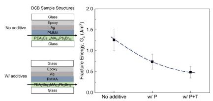
Fig. 6 The measured  $G_c$  values as a function of the incorporation of small molecule additive phosphine oxide (P) and tocylate (T) in the perovskite layer.
