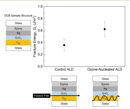
Fig. 3 A comparison between the average  $G_c$  results and fracture paths of control ALD-SnO<sub>x</sub> and Ozone-nucleated ALD-SnO<sub>x</sub> samples.
