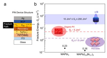
Fig. 2 (a) Device structure and fracture path. (b) The measured average  $G_c$  of the p-i-n samples with MAPbI<sub>3</sub> and MAP(I<sub>0.9</sub>Br<sub>0.1</sub>)<sub>3</sub> in comparison with the  $G_c$  of various PV technologies
