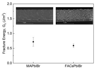
Fig. 4 The measured  $G_c$  of vacuum-evaporated MAPb( $I_{0.9}Br_{0.1}$ )<sub>3</sub> and FA<sub>0.74</sub>Cs<sub>0.26</sub>Pb(I<sub>0.86</sub>Br<sub>0.14</sub>)<sub>3</sub> perovskites (inset: cross-sectional SEM image of the perovskite laver)
