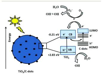
Fig. 4 The mechanism of photocatalytic degradation by CD/TiO<sub>2</sub>. Reproduced with permission.<sup>34</sup> Copyright 2018, RSC.
