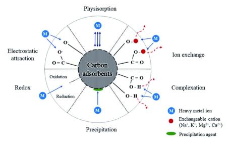
Fig. 3 Adsorption mechanism of carbon adsorbents. Reproduced with permission.<sup>27</sup> Copyright 2022, RSC.
