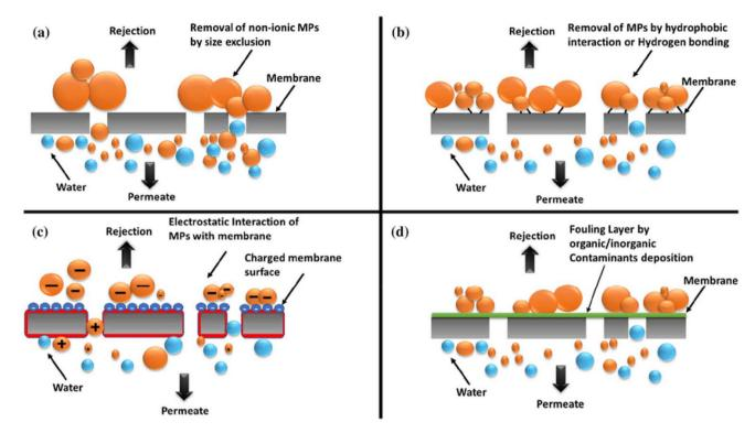
Fig. 5 Membrane filtration mechanisms—(a) size exclusion, (b) hydrophobicity, (c) electrostatic interaction, and (d) adsorption. Reproduced with permission.<sup>35</sup> Copyright 2020, Elsevier.
