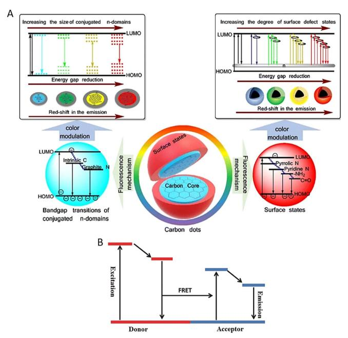
Fig. 2 (A) Fluorescence mechanism of CDs. Reproduced with permission.<sup>17</sup> Copyright 2019, Springer. (B) Mechanism of Förster Resonance Energy Transfer (FRET). Reproduced with permission.<sup>19</sup> Copyright 2017, Wiley
