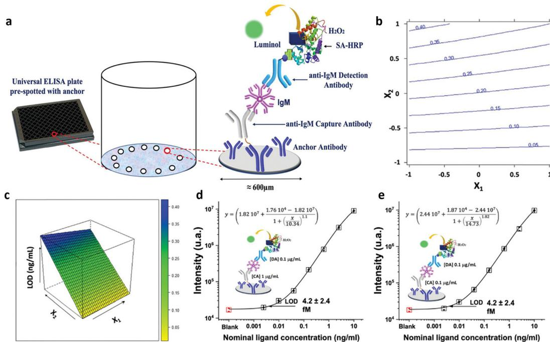
Fig. 4 (a) Scheme of the biosensor development; (b) isoresponse contour plot and (c) the response surface for LOD response. IgM calibration curve recorded using (d)  $1\ \mu\text{g mL}^{-1}$  and  $0.1\ \mu\text{g mL}^{-1}$  and (e)  $0.1\ \mu\text{g mL}^{-1}$  and  $0.1\ \mu\text{g mL}^{-1}$  of CA and DA anti-IgM antibodies respectively. Adapted and reproduced with permission from ref. 35. Copyright 2022, Wiley-VCH under Creative Commons Attribution 4.0 License (CC BY 4.0).
