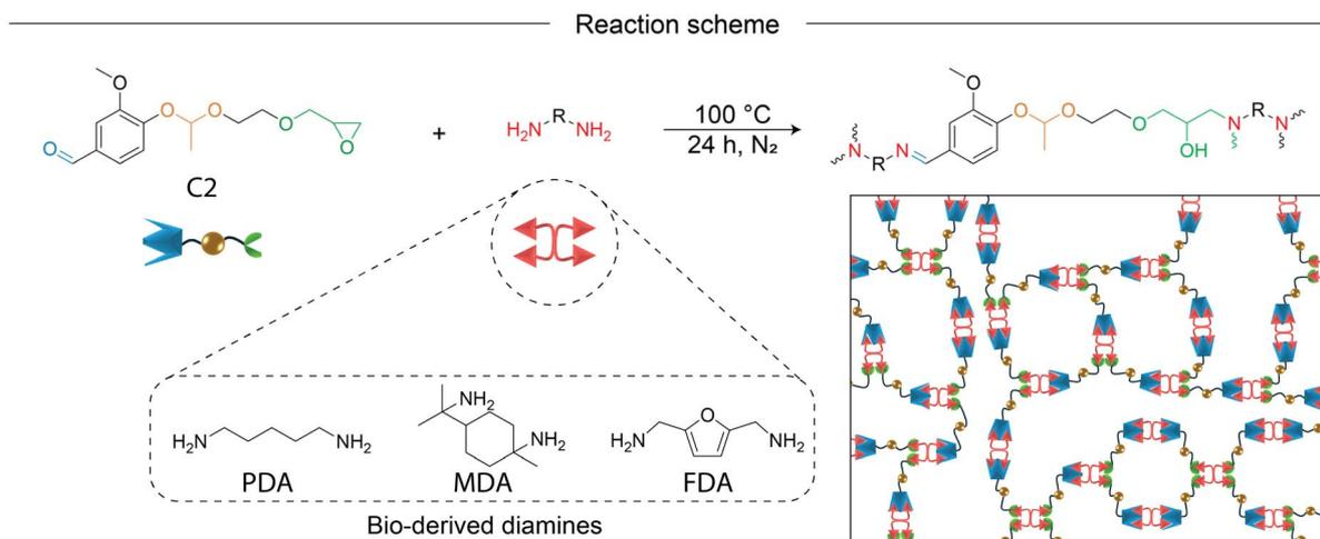
Scheme 1 Synthesis of bio-based, doubly-cleavable epoxy networks.
