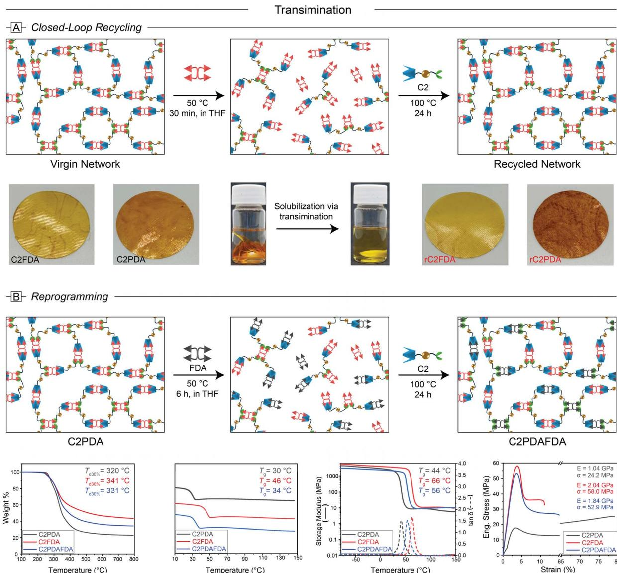
Fig. 4 (A) Illustrative representation of the closed-loop recycling concept *via* transimination, along with photographs of the original, solubilized, and recycled networks. (B) Synthesis of the C2PDAFDA network using the reprogramming approach, with comparative results from TGA, DSC, DMA, and tensile tests.
