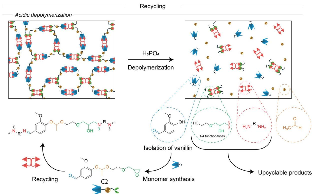
Fig. 3 Illustration of the recycling of designed epoxy networks utilizing controlled acidic depolymerization with 1 M H<sub>3</sub>PO<sub>4</sub> solution.
