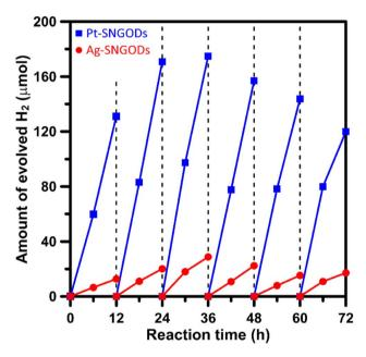
Fig. 3 Evolution of H<sub>2</sub> from the xylose solutions containing Pt-SNGODs and Ag-SNGODs under simulated solar irradiation (AM 1.5, 100 mW cm<sup>-2</sup>).
