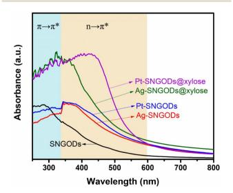
Fig. 1 Optical absorption spectra of the aqueous suspensions of SNGODs, Pt-SNGODs, Ag-SNGODs, Pt-SNGODs@xylose, and Ag-SNGODs@xylose. The absorption was arisen from the  $\pi \to \pi^*$  and n  $\rightarrow \pi^*$  transitions
