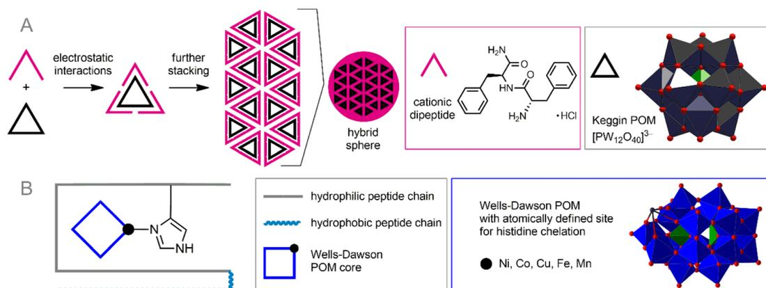
Fig. 3 Formation of nanoassemblies of anionic POMs with cationic peptides under the influence of electrostatic forces (A) and the synergetic effect of coordination bonds and electrostatic forces (B).
