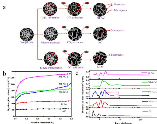
Fig. 3 (a) Schematic depiction of coal-based activated carbon preparation via melt permeation-assisted  $\text{CO}_2$  activation; (b)  $\text{N}_2$  adsorption/desorption isotherms of the prepared activated carbons; (c) corresponding DFT pore size distributions of the prepared activated carbons.<sup>68</sup>
