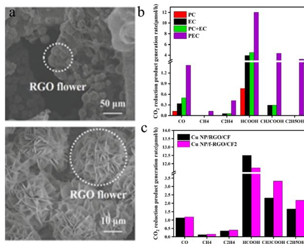
Fig. 10 (a) SEM images of the Cu NP/f-RGO/CF electrode (at different resolutions); (b) CO<sub>2</sub> reduction product generation rates on Cu NP/f-RGO/CF electrodes in a Pt-TNT photoanode-driven PEC cell under PC, EC, or PEC conditions. The voltage applied through the cell was 2 V under EC and PEC conditions; (c) CO<sub>2</sub> reduction product generation rates on the Cu NP/f-RGO/CF and Cu NP/RGO/CF cathodes in a Pt-TNT photoanode-driven PEC cell.<sup>115</sup>
