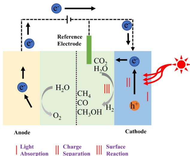
Fig. 9 Schematic diagram of the photoelectric catalysis of CO<sub>2</sub> reduction.<sup>110</sup>
