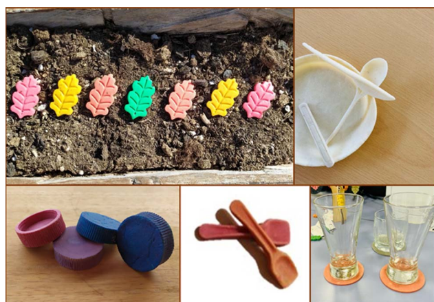
Fig. 8 Prototypes of commonly used items obtained from the LF/IGmix composite material.
