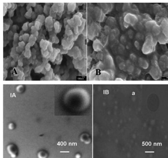
Fig. 4 SEM images of PDA-Lac- $\text{Fe}_3\text{O}_4$  (A) and PDA-Lac (B). This figure has been reproduced from ref. 31 with permission from Elsevier B.V., copyright 2012. (IA) SEM and (IB) TEM images of peroxalate polymer nanoparticles. This figure has been reproduced from ref. 42 with permission from Elsevier B.V., copyright 2012.
