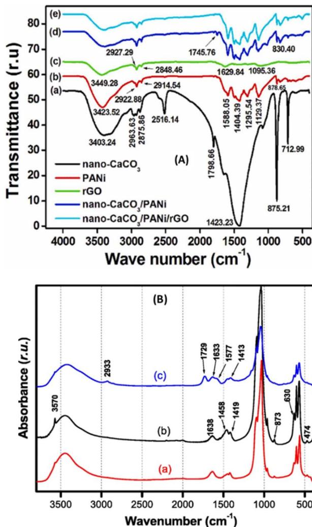
Fig. 2 (A) FTIR spectra of (a) nano-CaCO<sub>3</sub>, (b) PANi, (c) rGO, (d) nano-CaCO<sub>3</sub>/PANi, and (e) nano-CaCO<sub>3</sub>/PANi/rGO. This figure has been reproduced from ref. 23 with permission from Elsevier Ltd., copyright 2022. (B) FTIR spectra of (a) NHAP, (b) NHAPP0.5, and (c) NHAPP0.5-CA-β-CD materials. This figure has been reproduced from ref. 40 with permission from Springer-Verlag GmbH Germany, copyright 2021.
