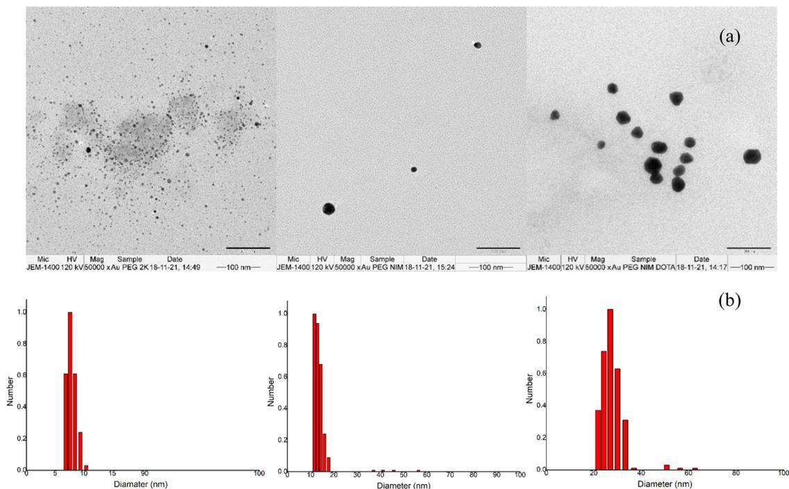
**Fig. 3** (a) TEM images of AuNP-PEG-2K-NH<sub>2</sub>, AuNP-PEG-2K-(2-NIM) and AuNP-PEG-2K-(2-NIM)(DOTA) [left to right]. (b) Size distribution data of AuNP-PEG-2K-NH<sub>2</sub>, AuNP-PEG-2K-(2-NIM) and AuNP-PEG-2K-(2-NIM)(DOTA) [left to right].
