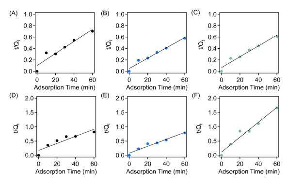
Fig. 7 Model fits to a pseudo-second order kinetic model for the adsorption of methylene blue by (A) the virgin EVA-derived sorbent, (B) Brand 1-derived sorbent, and (C) Brand 2-derived sorbent. Model fits to a pseudo-second order kinetic model for the adsorption of crystal violet by (D) the virgin EVA-derived sorbent, (E) Brand 1-derived sorbent, and (F) Brand 2-derived sorbent.
