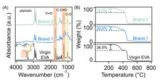
**Fig. 2** (A) FTIR spectra and (B) TGA thermograms of the EVA copolymer and waste shoe soles. The FTIR and TGA results are vertically shifted for clarity.
