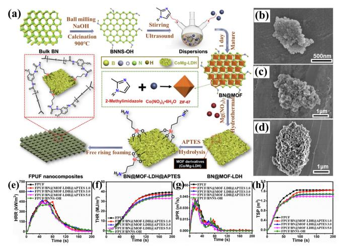
Fig. 12 (a) Preparation flow of BN@MOF-LDH@APTES nanohybrids; SEM images of (b) BN@MOF, (c) BN@MOF-LDH and (d) BN@MOF-LDH@APTES; (e) HRR, (f) THR, (g) SPR and (h) TSP curves of FPUF and its composites. Reproduced with permission from ref. 93, copyright reserved Elsevier 2022.
