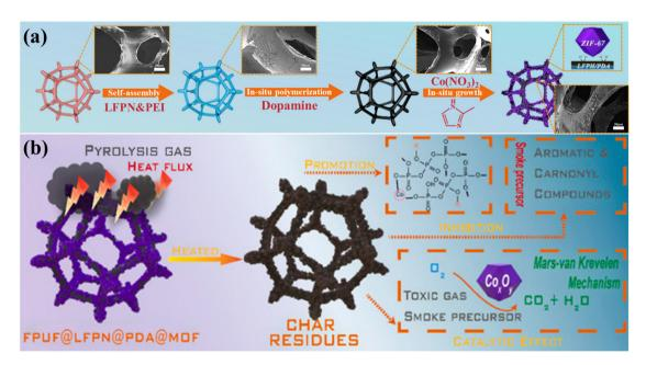
Fig. 10 (a) Preparation process and (b) flame retardant mechanism of FPUF@LFPN@PDA@MOF. Reproduced with permission from ref. 88, copyright reserved Elsevier 2024.
