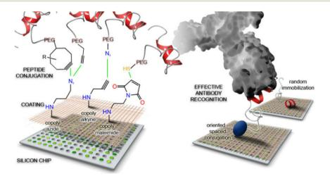
Fig. 14 Schematic illustration of peptide conjugation onto a 'clickable' polymer-coated silicon chip for effective antibody recognition. Adapted with permission from Gori et al. 108 Copyright © 2016 American Chemical Society.
