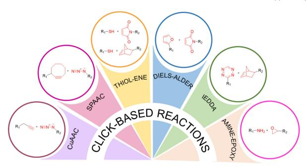
Fig. 2 Click-based reactions commonly utilized for fabricating functional polymeric interfaces.
