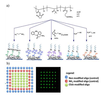
Fig. 15 (a) Fabrication of clickable polymer coatings via post-polymerization modification for microarray technology and (b) schematic representation of the oligonucleotides immobilized on the surfaces, coated with the 'click' copolymers. Adapted with permission from Sola et al. 109 Copyright © 2016 American Chemical Society.
