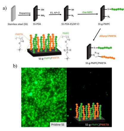
Fig. 6 (a) Schematic illustration of fabricating binary polymer brush coatings on stainless steel surfaces via 'click' reaction; (b) fluorescence microscopy images of pristine SS and SS-q-PMPC/PMETA brushes after exposure to S. aureus. Adopted with permission from Xu et al. 34 Copyright © 2017 American Chemical Society.
