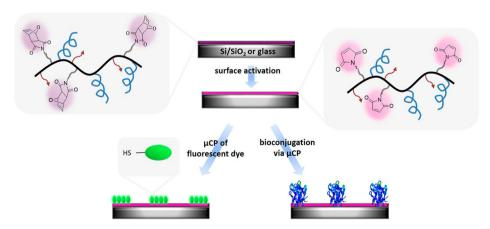
Fig. 16 Fabrication of a thiol-reactive polymer-based thin film coating for sensing and biomolecule immobilization. Adapted with permission from Gevrek et al. 127 Copyright © 2017 American Chemical Society.
