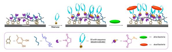
Fig. 9 Schematic illustration of an AMP-conjugated thiol-reactive polymeric coating on a TiO<sub>2</sub> surface to fabricate an antimicrobial coating. Adapted with permission from Gevrek *et al.*<sup>51</sup> Copyright © 2019 American Chemical Society.
