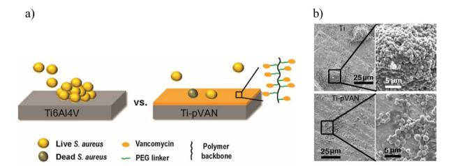
Fig. 10 (a) Fabrication of a vancomycin conjugated polymer brush on a titanium alloy for suppression of *S. aureus* colonization; (b) SEM of *S. aureus* adhered on unmodified  $Ti_6Al_4V$  and Ti-pVAN plates after 5 h incubation with  $1.2 \times 10^5$  CFU per mL *S. aureus*. Adapted with permission from Zhang et al. 60 Copyright © 2019 American Chemical Society.
