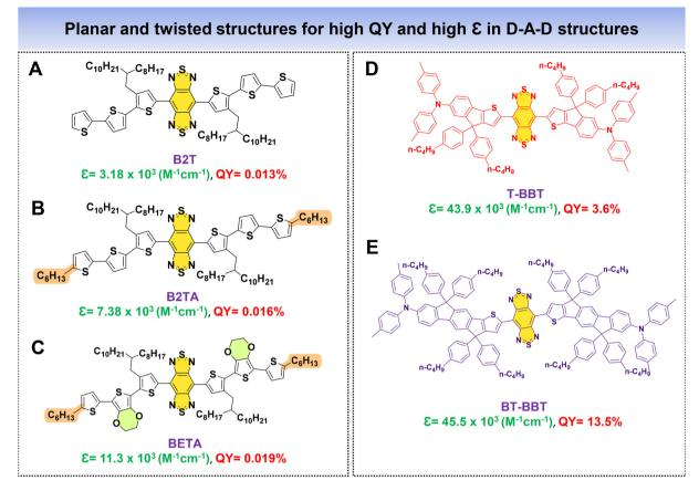
Fig. 11 D-A-D based fluorophores (A-E) with planar and twisted molecular architectures for high QY and high  $\varepsilon$ .
