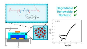
Fig. 8 Schematic representation of a degradable and biocompatible ion gels from a renewable ABA triblock polyester and ionic liquid. Reproduced from ref. 73 with permission from ACS, Copyright [2017].
