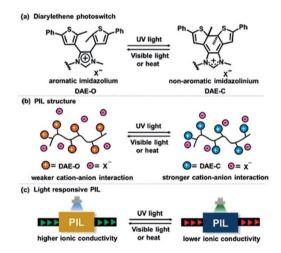
Fig. 51 (a) Photochromism of imidazolium-bearing DAE; (b) scheme of PIL with photoresponsive cation anion interaction; (c) solid-state PIL film with tunable, photoresponsive ionic conductivity. Reproduced from ref. 231 with permission from Wiley-VCH, Copyright [2020].
