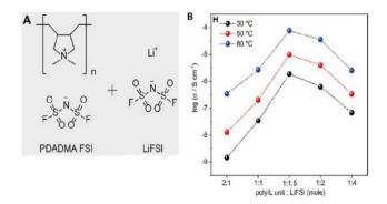
Fig. 34 (A) The chemical structures of poly(diallyldimethylammonium) bis(fluorosulfonyl)imide (PDADMA FSI) and Li bis(fluorosulfonyl)imide (LiFSI) salt. (B) The ion conductivities of different polyIL/salt systems at 30 °C, 50 °C, and 80 °C, respectively. The highest conductivity of 0.7  $\times$ 10<sup>4</sup> S cm<sup>-1</sup> is achieved for the 1:1.5 system at 80 °C. Reproduced from ref. 214 with permission from Elsevier, Copyright [2019].
