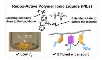
Fig. 53 Schematic structure of redox polymers with tethered chains inserted in between the backbone and pendants to target for low  $T_{q}$ charge conducting polymers. Reproduced from ref. 233 with permission from ACS, Copyright [2021].
