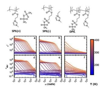
Fig. 67 Schematic representation of the polymers investigated in the study. Frequency dependence of (a–c) the dielectric permittivity and (d–f) the dielectric loss derivative function  $\varepsilon_{\rm der}$  for (a and d) SPIL(+), (b and e) SPIL(–), and (c and f) DPIL across the range of temperatures investigated in the study. Reproduced from ref. 22 with permission from ACS, Copyright [2021].
