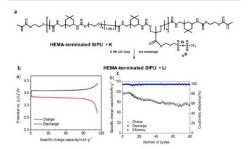
Fig. 31 (a) Schematic representation of the polyurethane-based polymer investigated in the current study. (b) Lithium metal/XSIPU-PC/ LiFePO $_4$  cell potential *versus* specific discharge capacity at C/10 and ambient temperature; (c) specific capacity *versus* cycle number. Reproduced from ref. 211 with permission from Elsevier, Copyright [2017].
