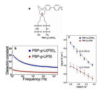
Fig. 60 (a) Schematic representation of grafted poly(biphenyl piperidinium)s including PBP-g-Li(PSI)<sub>2</sub> (b) dielectric spectra of PBP-g-Li(PSI)<sub>2</sub> and PBP-q-LiPSI (c) ionic conductivity of PBP-q-LiPSI and PBP-q-Li(PSI)<sub>2</sub> gel blend polymer electrolyte membranes. Reproduced from ref. 247 with permission from Elsevier, Copyright [2022].
