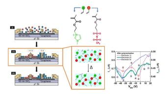
Fig. 66 Schematic representation of ion-locking phenomenon in [EMIM][TFSI]-modeled DPIL to create a stable p-n junction in a two-dimensional semiconductor. The resulting transfer characteristics of a representative device are shown here; the presence of two current minima with variation in the back gate voltage are the tell-tale signature of successful formation of a p-n junction. Reproduced from ref. 21.
