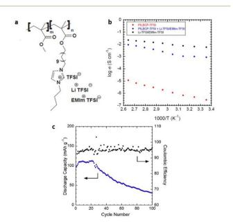
Fig. 29 (a) Schematic representation of the PILBCP-TFSI polymer. (b) Temperature-dependent dry ionic conductivity of PILBCP-TFSI (red), PILBCPTFSI + Li-TFSI/EMIm-TFSI (blue), and Li-TFSI/EMIm-TFSI (black). (c) Discharge capacity and coulombic efficiency as a function of cycle number and (b) rate is 0.1 C. Reproduced from ref. 209 with permission from Elsevier, Copyright [2016].
