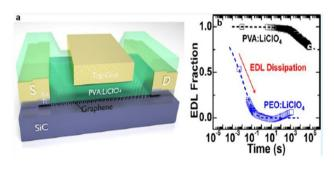
Fig. 65 (a) Schematic representation of the graphene FET fabricated; (b) enhancing the room-temperature electric double layer retention time in 2-D crystal FETs. Reproduced from ref. 251 with permission from ACS, Copyright [2017].
