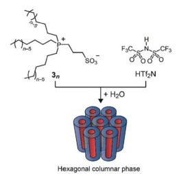
Fig. 14 Zwitterionic compounds 3n consisting of a phosphonium cation and a sulfonate anion. An equimolar mixture of 3n and HTf2N forms a homogeneous complex that exhibits lyotropic columnar liquid crystalline phases in the presence of water. Reproduced from ref. 104 with permission from RSC, Copyright [2011].
