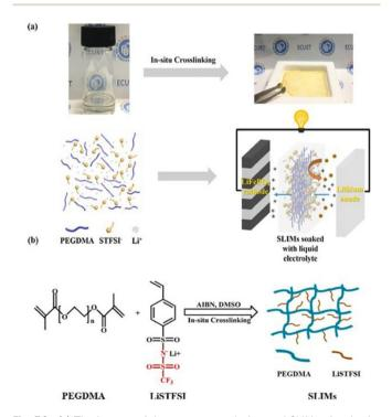
Fig. 36 (a) The images of the precursor solution and SLIMs after in situ crosslinking, with the corresponding change of structures. (b) Preparation process of SLIMs by in situ crosslinking reaction. Reproduced from ref. 216 with permission from Elsevier, Copyright [2020].
