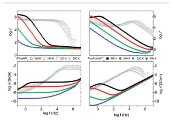
Fig. 22 The complex dielectric function  $\varepsilon^*(\varepsilon'-i\varepsilon'')$  and the complex conductivity function  $\sigma^*(\sigma'+i\sigma'')$  versus frequency at different temperatures as indicated for the polymerized ionic liquid (poly(PVIM) NTf<sub>2</sub>) (closed symbols) and the corresponding low molecular weight ionic liquid (open symbols) at selected temperatures. Reproduced from ref. 20 with permission from RSC, Copyright [2014].
