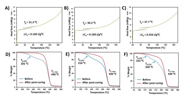
Fig. 5 DSC analysis showing the second heating curves used to determine the glass-transition temperatures and heat capacities of: (A) the DAS: PEGDA sample; (B) the DAM: PEGDA sample; and (C) the DAT: PEGDA sample. TGA curves, illustrating the main degradation steps, before and after complete curing, for: (D) the DAS: PEGDA sample; (E) the DAM: PEGDA sample; and (F) the DAT: PEGDA sample.
