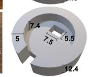
Fig. 2 (A) 3D model of heating plate enclosure. (B) Dimensions of coin cell battery holder. (C) 3D models of top and bottom of battery enclosure.
