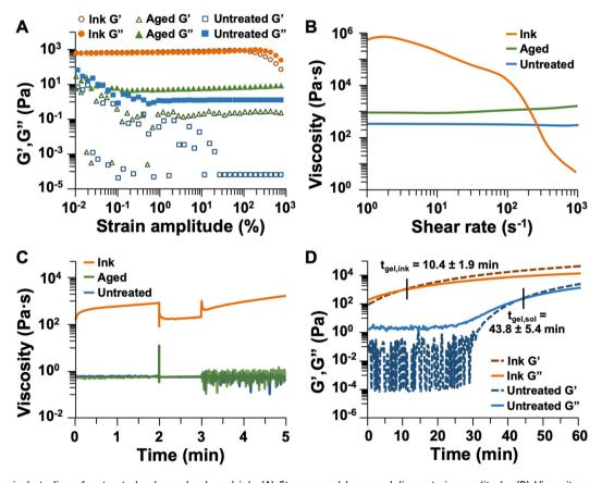
Fig. 6 Rheological studies of untreated sol, aged sol, and ink. (A) Storage and loss moduli vs. strain amplitude. (B) Viscosity vs. shear rate. (C) Viscosity vs. time during three-interval thixotropy test. (D) Storage and loss modulus vs. time during gel point measurement for untreated sol and
