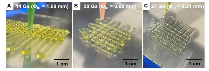
Fig. 5 Photographs showing direct ink writing of aerogel lattices using different nozzle sizes (A) 14 Ga, (B) 20 Ga, (C) 27 Ga.
