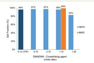
**Fig. 3** The gel fractions of p(DMAEMA-co-BMA) (50:50 mole ratio) crosslinked with DBPO and BBEE. Gel fractions were determined by Soxhlet extraction in refluxing THF for 1 week.
