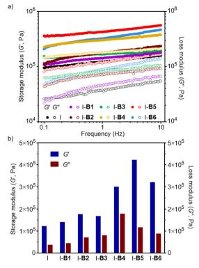
Fig. 8 (a) Storage (G') and loss moduli (G'') of the ionomer, I-B1, B2, B3, **B4**, **B5** and **B6** measured by frequency sweeps at 70 °C. (b) G' and G" of the ionomer, I-B1, B2, B3, B4, B5 and B6 at 1 Hz.
