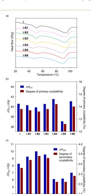
Fig. 4 (a) DSC curves of the ionomer and samples from I-B1 to I-B6 at a scanning rate of 10 °C min<sup>-1</sup>. (b) Heat of fusion ( $\Delta H_{m1}$ ) and degree of primary crystallinity (%) and (c) heat of fusion ( $\Delta H_{m2}$ ) and degree of secondary crystallinity (%) of the ionomer and I-B1 to I-B6.
