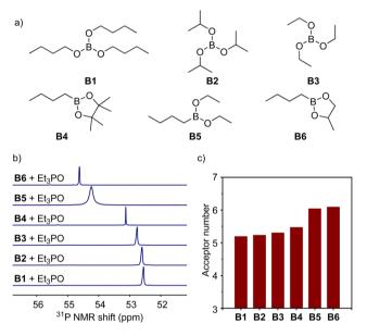
Fig. 2 (a) Chemical structures of boron compounds studied in this work (B1 to B6). (b) <sup>31</sup>P NMR results of Et<sub>3</sub>P=O in the presence of boron compounds. (c) Acceptor numbers of boron compounds determined by the Gutmann-Beckett method.
