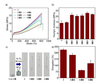
Fig. 6 (a) Stress-strain curves and (b) Young's modulus of the ionomer (I) and samples from I-B1 to I-B6 measured at 70 °C. (c) Optical images and (d) results of the elongation experiments of the ionomer, I-B3, I-B5 and I-B6 conducted at 75 °C.
