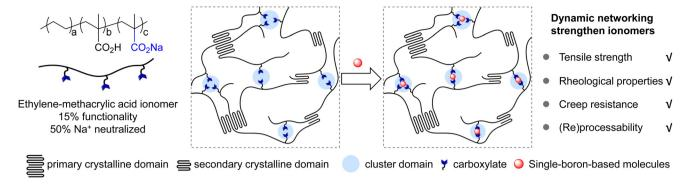
Fig. 1 Structure and physical interactions of the unmodified and modified ionomers.
