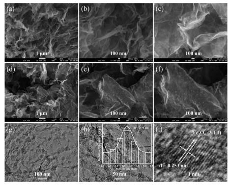
Fig. 3 FESEM images of Fe-BTC/TP-RGO (a-c) and Fe<sub>3</sub>O<sub>4</sub> QDs@C/RGO (d-f) samples under various magnifications. TEM images (g and h) of the Fe<sub>3</sub>O<sub>4</sub> QDs@C/RGO sample under different magnifications with inset showing Fe<sub>3</sub>O<sub>4</sub> particle size distribution. HRTEM image (i) for an individual Fe<sub>3</sub>O<sub>4</sub> nanoparticle in the Fe<sub>3</sub>O<sub>4</sub> QDs@C/RGO sample.
