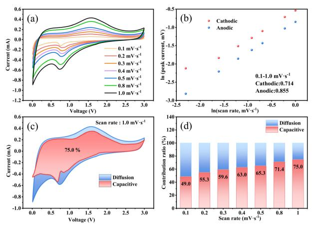
Fig. 5 CV curves of the Fe<sub>3</sub>O<sub>4</sub> QDs@C/RGO composite electrode from 0.1 to 1.0 mV s<sup>-1</sup> (a), the  $\ln(i)$ - $\ln(v)$  plot (b), the capacitive contribution of the Fe<sub>3</sub>O<sub>4</sub> QDs@C/RGO composite electrode at 1 mV s<sup>-1</sup> (c) and the pseudocapacitive contribution ratios at different scanning rates (d).
