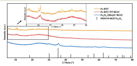
Fig. 1 XRD patterns of the Fe-BTC, Fe-BTC/TP-RGO and Fe<sub>3</sub>O<sub>4</sub> QDs@C/RGO samples
