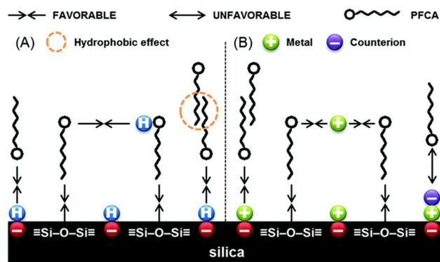
**Fig. 1** Possibly enhanced perfluorocarboxylic acid (PFCA) aggregation through solute–silica and solute–solute H-bonding at low pH (A), and anion shielding by background electrolytes (B) reprinted from ref. 5. Copyright 2017 RSC.
