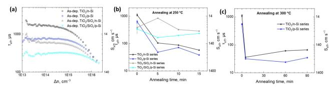
Fig. 2 (a) Injection-level dependent effective lifetimes for Si wafers passivated by 54 nm thin films of (a) as-deposited TiO2, (b) annealed TiO2 films at 250 °C, and (c) annealed TiO<sub>2</sub> films at 300 °C for different durations. The corresponding surface recombination velocities ( $S_{eff}$ ) are also shown on the right y-axis.
