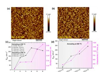
Fig. 7 AFM images of (a) as-dep. TiO<sub>2</sub>/n-Si, (b) 90 min annealed TiO<sub>2</sub>/n-Si at 300 °C, (c) correlation of surface recombination velocity and surface roughness of the samples, and (d) correlation of surface recombination velocity and characteristic charge transfer times for HF-treated TiO<sub>2</sub>/n-Si heterojunctions annealed at 250 °C up to 15 minutes
