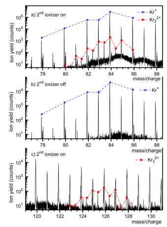
Fig. 1 A mass spectrum of HNDs doped with Kr reveals the existence of  $Kr_2^{2+}$  and  $Kr_3^{2+}$  when both ionizers are turned on (panels a and c, respectively). The expected abundance distributions of their isotopologues are indicated by dash-dotted lines. Only singly charged Kr ions are seen when the second ionizer is turned off (panel b)
