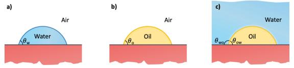
Fig. 2 Sessile droplets on a solid surface. (a) Water droplet in air, characterized by the water (w) contact angle θ<sub>w</sub>. (b) Oil droplet in air, characterized by the oil (o) contact angle  $\theta_{o}$ . (c) Oil droplet in water, characterized by the oil-in-water (o/w) contact angle  $\theta_{ow}$ . The latter is related to the water-in-oil (w/o) contact angle  $\theta_{\rm wo}$  via the relation  $\theta_{\rm wo}$  +  $\theta_{\rm ow}$  = 180°.
