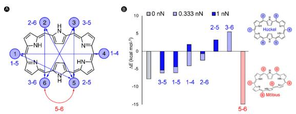
Fig. 7 (A) Numbering of the meso-positions of the [28]hexaphyrin macrocycle. Pulling scenarios promoting the Hückel (in blue) or the Möbius (in red) conformation, based on the distance matrices. (B) Energies of the Möbius structure relative to the Hückel topology for different force regimes. A positive sign indicates a more stable Hückel structure, whereas a negative sign means the opposite.
