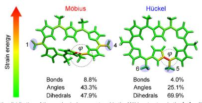
Fig. 8 JEDI analysis showing the distribution of the mechanical energy stored in the Möbius structure in the 1-4 pulling scenario at 1.0 nN and the Hückel structure in the 5-6 pulling scenario at 0.333 nN. Circular contours highlight the most activated regions by the external force and correspond to the reaction coordinate triggering the topology interconversions. Reprinted from Chemistry - A European Journal, ref. 32.
