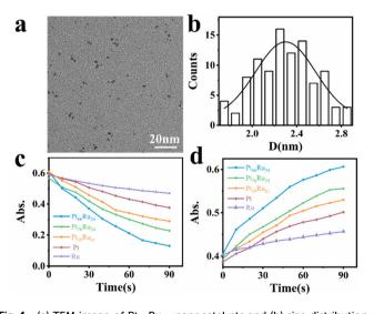
Fig. 1 (a) TEM image of  $Pt_{66}Ru_{34}$  nanocatalysts and (b) size distribution of  $Pt_{66}Ru_{34}$  nanoparticles with an average of about 2.3  $\pm$  0.03 nm. Dependence of (c) 601 nm and (d) 571 nm absorbance on time for nanocatalysts with different ratios. All of the experiments were carried out in a saturated  $H_2$  solution with the same nanoparticle concentration and resazurin concentration.
