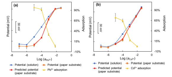
Fig. 3 Corrective protocol to predict interference free sensor response of ISE coupled with paper-based microfluidic solution sampling from solution-based measurement of (a)  $Pb^{2+}$  and (b)  $Cd^{2+}$ -ISEs.
