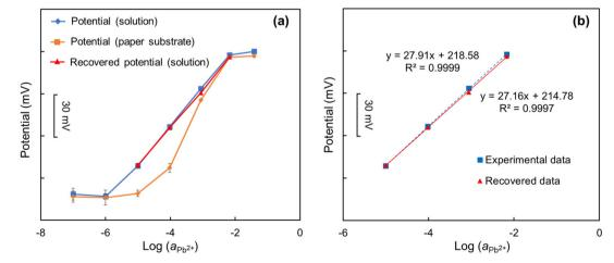
Fig. 6 Corrective protocol to predict interference free sensor response from the paper-based potential in case 2: (a) calibration curves of the fabricated Pb<sup>2+</sup> ISEs on paper substrate, on standard mixed solution and recovered solution-based calibration curve from paper-based calibration curve; (b) slopes and linearities of the experimental solution-based calibration curve and the recovered solution-based calibration curve.
