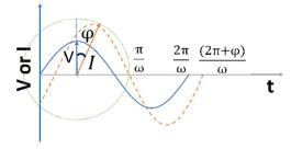
Fig. 2 The alternating current exhibits a sinusoidal response to the applied voltage waveform at an angular frequency of  $\omega$  in a linear
