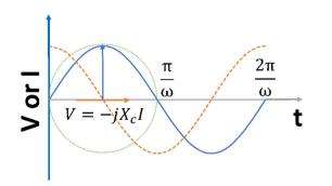
Fig. 4 The current generated when a sinusoidal potential is applied to a pure capacitance.
