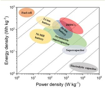
Fig. 1 Ragone plot of Zn-ion hybrid supercapacitors (ZIHSCs) comparing their performance with other standard energy storage systems (ESSs)
