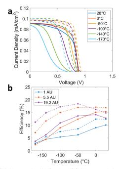
Fig. 6 (a) J-V curves for ANU9 cell at 19.2 AU post-radiation, with preradiation J-V curves shown in dotted lines. (b) Post-radiation efficiency of the ANU9 cell with respect to temperature at various light intensities, with pre-radiation efficiencies shown in dotted lines
