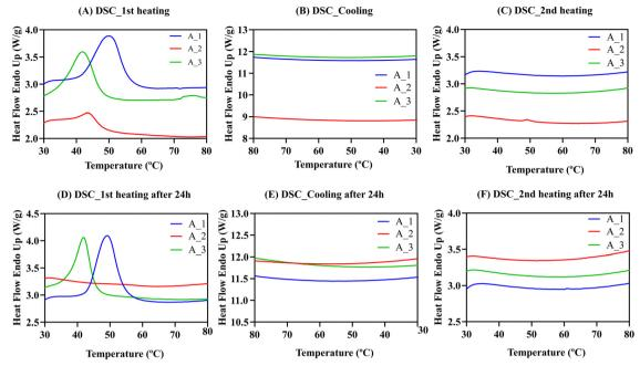
Fig. 9 (A) First heating DSC scans for hydrogel A. A\_1 empty hydrogel A. A\_2 hydrogel A with BSA. A\_3 hydrogel A with BSA-FITC. (B) DSC cooling scans. (C) Second heating DSC scans. (D) First heating DSC scans after 24 h. (E) DSC cooling scans for the second experiment. (F) Second heating DSC scans for the second experiment. Heating and cooling rates for all cases are 20  $^{\circ}$ C min<sup>-1</sup>
