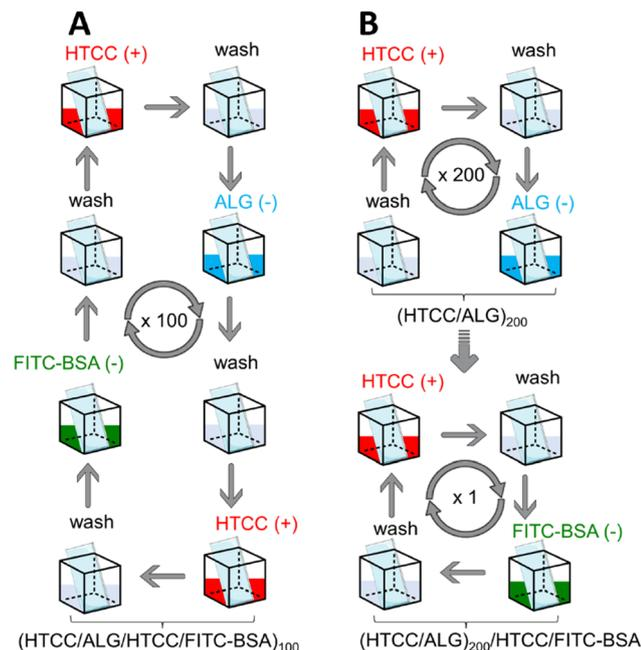
Fig. 1 Schematic illustration of the preparation of the two set-ups of FS multilayered membranes: (A) (HTCC/ALG/HTCC/FITC-BSA)<sub>100</sub> and (B) (HTCC/ALG)<sub>200</sub>/HTCC/FITC-BSA assembled onto poly(vinyl carbonate) substrates by resorting to attractive electrostatic interactions between HTCC, ALG and FITC-BSA.
