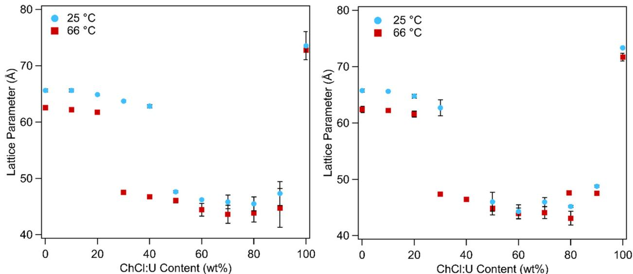
Fig. 10 Lattice parameters for 10 wt% (left) and 30 wt% (right) phytantriol as functions of ChCl:U content (wt%) at 25 and 66 °C. Lattice parameters above 60 Å are associated with the *Pn3m* cubic phase while lattice parameters below 60 Å are associated with the inverse hexagonal phase. Error bars are based on the standard deviation of multiple measurements and in some cases are smaller than the symbols.
