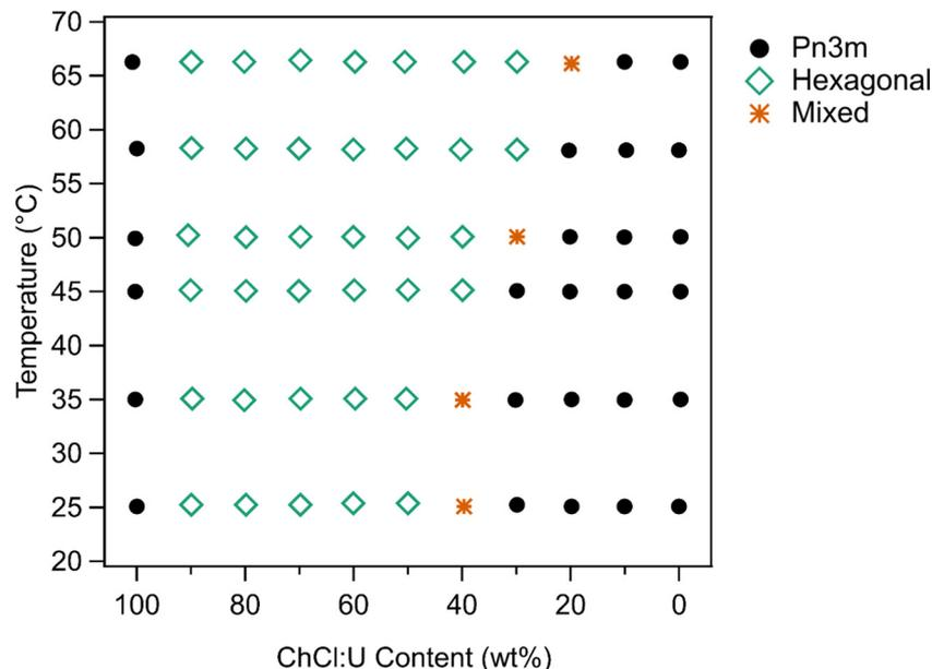
Fig. 6 Phase diagram of 10 wt% phytantriol as a function of ChCl:U/water% and temperature. The X-axis refers to the ChCl:U content in the solvent; the concentration of phytantriol is always 10 wt% with 90 wt% solvent.
