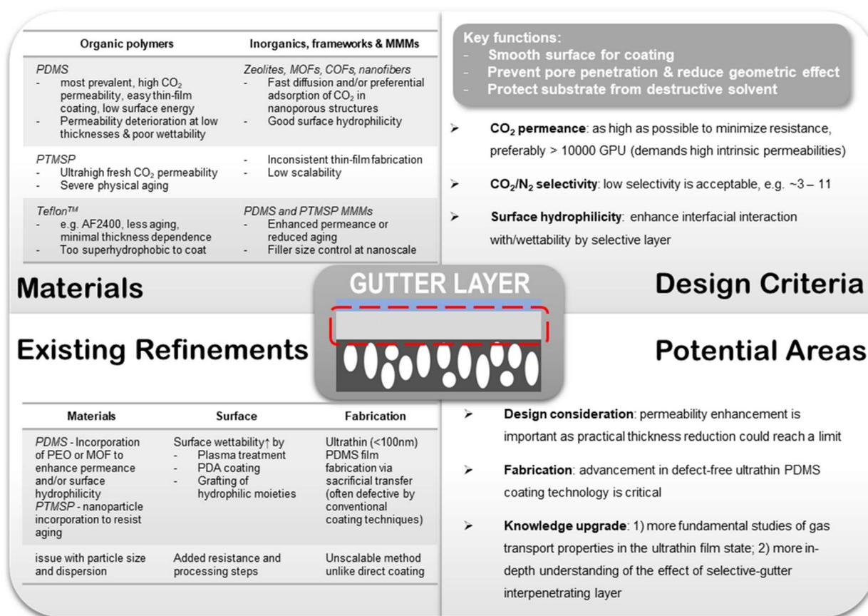
Fig. 7 Design summary for the gutter layer.
