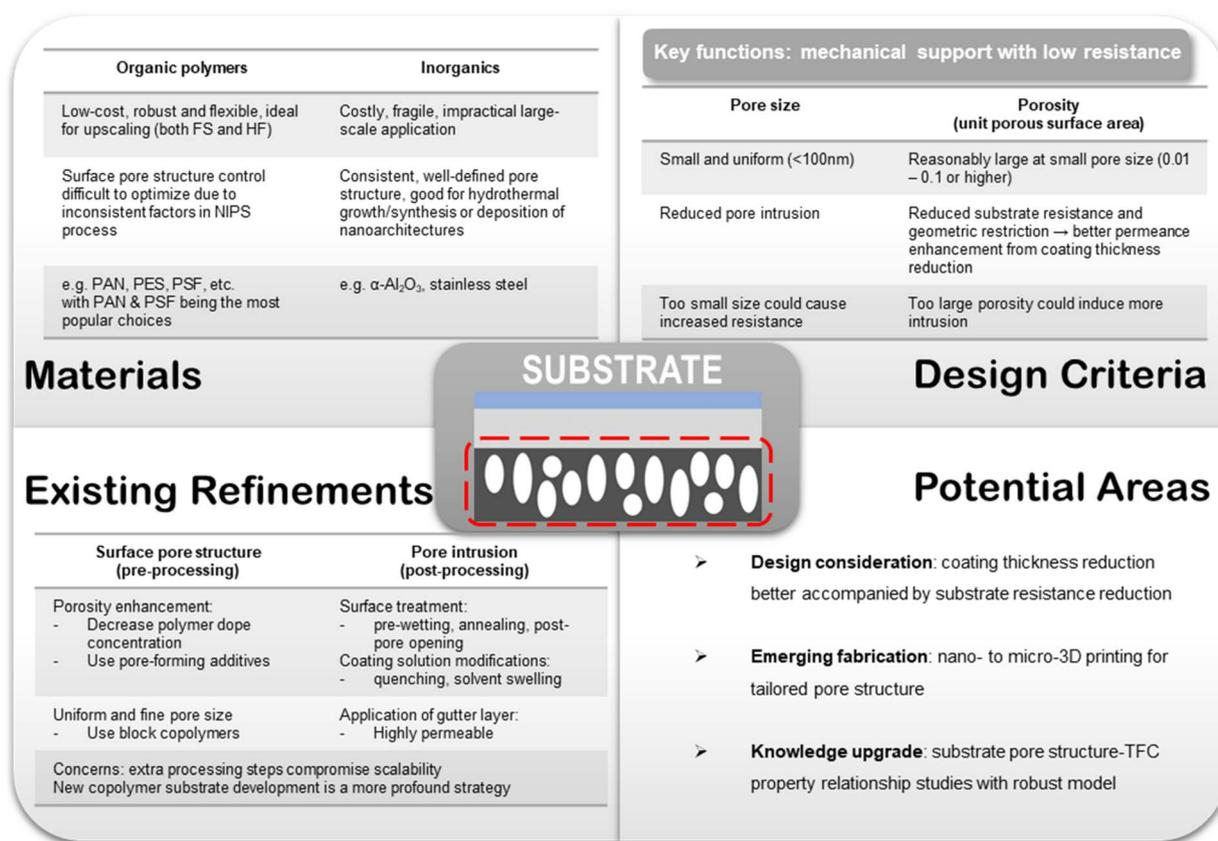
Fig. 6 Design summary for the porous substrate layer.
