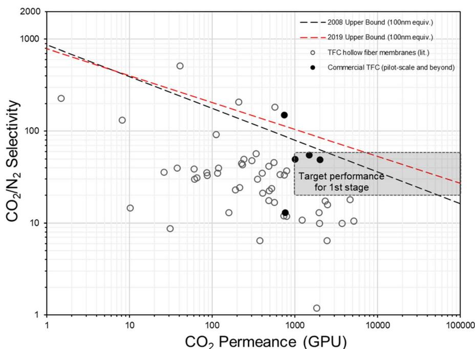
Fig. 11 Summary of the CO<sub>2</sub>/N<sub>2</sub> separation performance of existing representative TFC hollow fiber membranes against the hypothesized thin-film upper bounds (assuming 100 nm thickness<sup>9,21,28</sup>) and proposed industrial targets.
