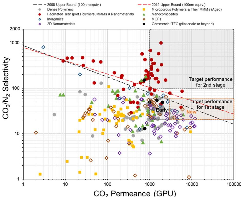
Fig. 4 Summary of the CO<sub>2</sub>/N<sub>2</sub> separation performance of existing representative TFC membranes against the hypothesized thin-film upper bounds (assuming 100 nm thickness<sup>9,28</sup>) and proposed industrial targets.
