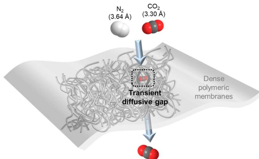
Fig. 1 Illustration of CO<sub>2</sub>/N<sub>2</sub> separation through a dense polymeric membrane.
