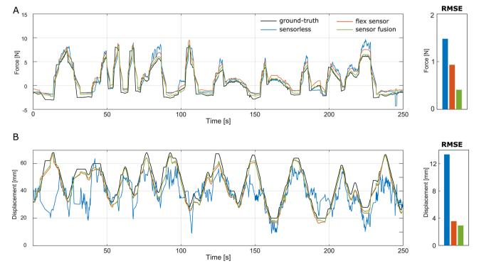
Fig. 7 Estimation results for pulling, along with root mean squared errors, using the three estimation strategies with previously unseen data. (A) Force estimation, (B) displacement estimation.
