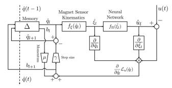
A block-diagram of the gradient descent as an iterative update loop for the configuration belief  $\hat{q}(t)$ . The gradient descent is initialized with the optimized solution  $\hat{q}_0 = \hat{q}(t-1)$  from the previous time-step. Note that during the iterative loop,  $\hat{q}_{l+1}$  updates  $\hat{q}_l$  in the memory block.
