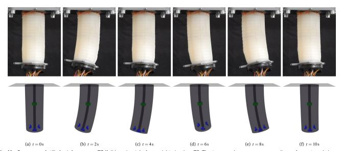
Fig. 11 Sequence of stills for inference on T3 (full lemniscate) of a model trained on T5. The top row shows camera recordings of an external view and the sequence in the bottom row consists of renderings of the ground-truth state (in full opacity) and the estimated segment shape (slightly transparent). The sensors are colored in blue and the ring magnet integrated into the backbone is shown in green.
