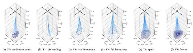
Fig. 9 Trajectories used during the experiments. We plot the shape of the segment under PCC approximation in light blue and the position of the tip of the segment in dark blue.
