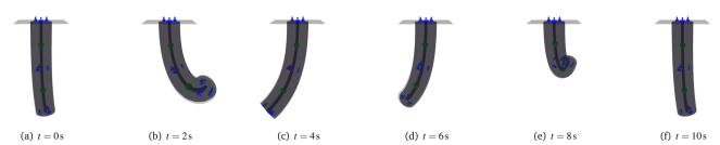
Fig. 7 Sequence of stills for a simulated affine curvature robot. We visualize the ground-truth shape of the soft robot with full opacity and the estimated configuration with slight transparency. The two magnets are rendered in green and the nine sensors in blue.
