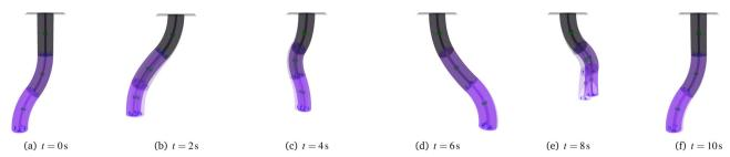
Fig. 5 Sequence of stills for simulated sensor failure as shown in Fig. 4(b): the number of sensors per segment, which are rendered in blue, is reduced from four to three at t = 5 s. We visualize the ground-truth shape of the soft robot with full opacity and the estimated configuration with slight transparency. The magnets are rendered in green and the three segments are visualized in a color sequence from black to violet.
