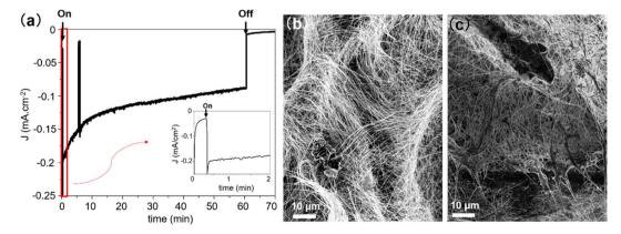
Fig. 7 (a) Chronoamperometry of PCS-SiNW-MoS<sub>x</sub> at -0.15 V vs. RHE in 0.5 M  $H_2$ SO<sub>4</sub> under illumination (48 nm-SiNWs,  $\Delta Q_{MoS_x} = 6$  mC cm<sup>-2</sup>) with N<sub>2</sub> bubbling. SEM images of the electrode before (b) and after (c) the stability test.
