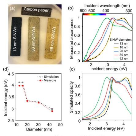
Fig. 3 Tuning SiNW absorption wavelength by their diameter: (a) photograph of PCS-SiNW. (b) Normalized spectra of measured absorption for SiNWs from PCS-SiNW with 13, 16, 20, 30 and 42 nm SiNWs. The rainbow indicates the visible range. (c) Normalized spectra of simulated opacity for TE polarization of SiNWs of diameters 13 to 42 nm (same legend as (b)). (d) Position of the plasmonic peak as a function of the SiNW diameter in measured and simulated spectra.
