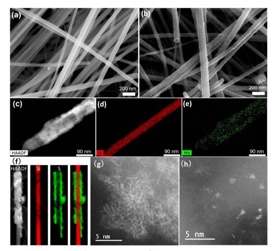
Fig. 4 SEM images of (a) 48 nm-SiNWs, (b) SiNW-MoS<sub>x</sub> with  $\Delta Q = 6$  mC cm<sup>-2</sup> (c) HAADF-STEM image of SiNW-MoS<sub>x</sub> and EDX mapping profile of (d)  $Si(K_{rg})$  and (e)  $Mo(K_{rg})$ ; (f) STEM-HAADF image and EELS mapping profile of element Si (L edge at 99 eV) and S (L edge at 165 eV); (g, h) Highresolution HAADF-STEM images of a-MoS<sub>x</sub>.
