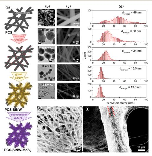
Fig. 2 Tuning SiNW diameter by the size of AuNPs: (a) scheme of the PCS-SiNW-MoS $_x$  photocathode fabrication. SEM and TEM images of the AuNPs of size 3–80 nm (b) and the subsequent SiNWs grown from them (c); (d) corresponding SiNW diameter histograms (>500 counts); SEM images of the PCS-SiNW (e) and close up view of a single carbon fiber (f). Red dotted lines highlight the diameter of the carbon fiber.
