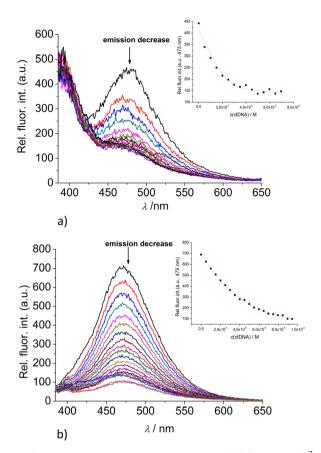
Fig. 5 Changes in the fluorescence spectra of: (a) 2 ( $c=5\times10^{-7}$  M) and (b) 3 ( $c=5\times10^{-7}$  M) upon titration with ctDNA ( $c=1\times10^{-3}$  M) at  $\lambda_{\rm exc}=350$  nm. (Insets) Dependence of 2 and 3 emission intensity at 475 nm on c(ctDNA). Done at pH 7.0, sodium cacodylate buffer, I=0.05 M.
