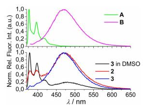
Fig. 2 (Top) 1-pyrenebutyric acid A ( $\lambda_{exc}=342$  nm) and peptide B ( $\lambda_{exc}=352$  nm) in water (0.01% DMSO). (Bottom) Normalised fluorescence spectra of 2 ( $\lambda_{exc}=352$  nm, water), 3 ( $\lambda_{exc}=350$  nm, water) and 3 ( $\lambda_{exc}=350$  nm, DMSO). Normalisation was performed by dividing a complete spectrum by the maximal intensity of emission.
