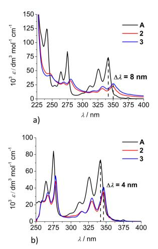
Fig. 1 Comparison of UV/Vis spectra: A (1-pyrenebutyric acid),  $^{36}$  2 and 3 at concentration  $c=1\times 10^{-5}$  M in: (a) water, (b) DMSO. The  $\Delta\lambda$  values are shown only for 342 nm maximum of A but bathochromic shift is present for complete spectra of 2 or 3.
