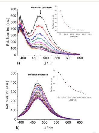
Fig. 4 Changes in the fluorescence spectra of: (a) **2** ( $c=5\times10^{-7}$  M) and (b) **3** ( $c=1\times10^{-6}$  M), upon titration with GMP ( $c=1\times10^{-3}$  M) at  $\lambda_{\rm exc}=350$  nm. (Insets) Dependence of **2** and **3** emission intensity at 475 nm on c(GMP). Done at pH 7.0, sodium cacodylate buffer, I=0.05 M.
