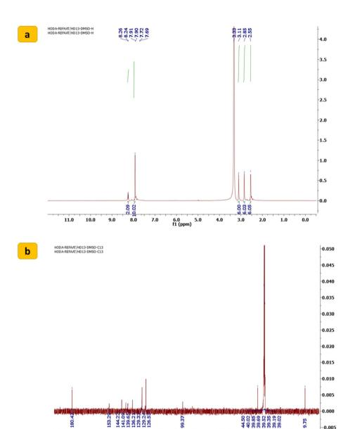
Fig. 2 (a)  $^{1}H$  NMR spectrum and (b)  $^{13}C$  NMR spectrum of 1,1'-((sulfonylbis(4,1-phenylene))bis(5-methyl-1H-1,2,3-triazole-1,4-diyl))bis(3-(dimethylamino)prop-2-en-1-one) (SBDMP) (2).
