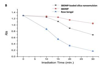
Fig. 10 Quenching of DPIBF (1 mM) at 420 nm. The absorbance (Abs) decreased with an increase in the irradiation time compared to the standard photosensitizer rose bengal (RB) over 30 min. DPIBF was oxidized by singlet oxygen photogenerated against (A) Syncephalastrum racemosum and (B) Rhizopus microsporous.
