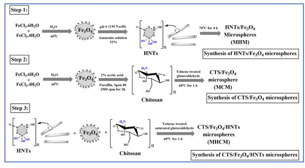
Fig. 1 Chemical scheme for the synthesis of microspheres (MHM, MCM, and MHCM), (step 1) synthesis of HNT magnetic microspheres (MHM) in the presence of an ammonia solution, (step 2) synthesis of CTS magnetic microspheres (MCM) in the presence of toluene-saturated glutaral-dehyde (TSG), and (step 3) synthesis of CTS and HNT magnetic microspheres (MHCM) with TSG.
