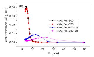
Fig. 4  $\rm N_2$  adsorption-desorption isotherms of the calcined (A) and spent (B) samples. Pore size distribution of the calcined (C) and spent (D) samples.
