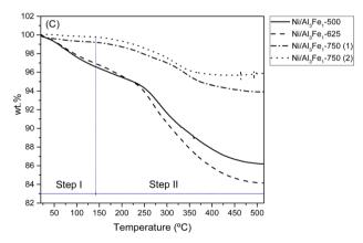
Fig. 5 XRD patterns of the calcined (A) and used (B) samples. TGA curves of the used samples (C). Step I: physisorbed water and step II: chemisorbed water and boehmite transformation.
