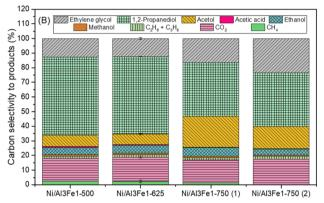
Fig. 2 Gas composition (vol%,  $N_2$ , and  $H_2O$  free) (A) and carbon selectivity to products (B).
