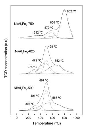
Fig. 6 H<sub>2</sub>-TPR profiles of the calcined samples.
