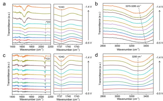
**Fig. 4** *In situ* attenuated total reflection surface-enhanced infrared absorption spectroscopy spectra of (a and b) Cu and (c and d) Cu-3TA catalysts in  $CO_2$ -saturated 0.1 M  $KHCO_3$  solution.
