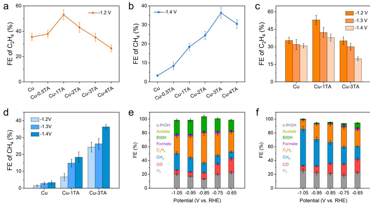
**Fig. 3** (a and b) Faradaic efficiency (FE) of  $C_2H_4$  and  $CH_4$  on Cu and Cu-xTA ( $x$  from 0.5 to 4) catalysts in  $CO_2$ -saturated 0.1 M  $KHCO_3$  solution in H-Cell. (c and d) FE of  $C_2H_4$  and  $CH_4$  on Cu, Cu-1TA and Cu-3TA catalysts under different potentials in H-Cells. (e and f) FE of products distribution on Cu-1TA and Cu-3TA catalysts at different applied potential in 1 M  $KHCO_3$  solution in flow cells.
