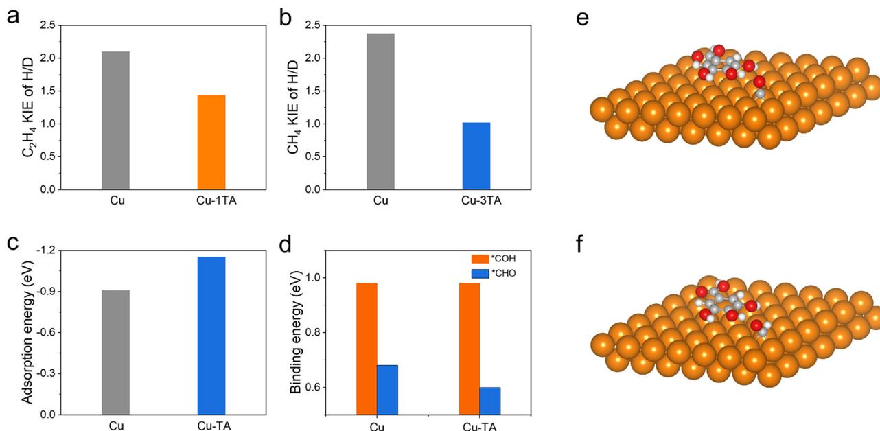
Fig. 5 (a) Kinetic isotope effect (KIE) value of C<sub>2</sub>H<sub>4</sub> on Cu and Cu-1TA catalysts at -0.85 V in a flow cell. (b) KIE value of CH<sub>4</sub> on Cu and Cu-3TA catalysts at -1.05 V in a flow cell. (c) Calculated adsorption energy of \*CO on Cu and Cu-TA catalysts. (d) Binding energy from \*CO to \*COH or \*CHO intermediate on Cu and Cu-TA catalysts. (e and f) Optimized adsorption configuration of \*CO and \*CHO intermediates on the Cu-TA catalyst.
