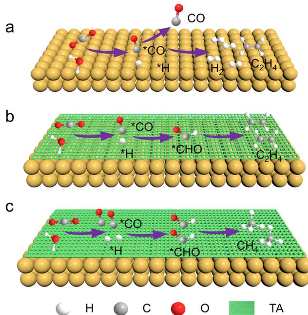
Fig. 1 Schematic illustration of CO<sub>2</sub>RR on the surfaces of (a) Cu, (b) Cu-1TA and (c) Cu-3TA catalysts.
