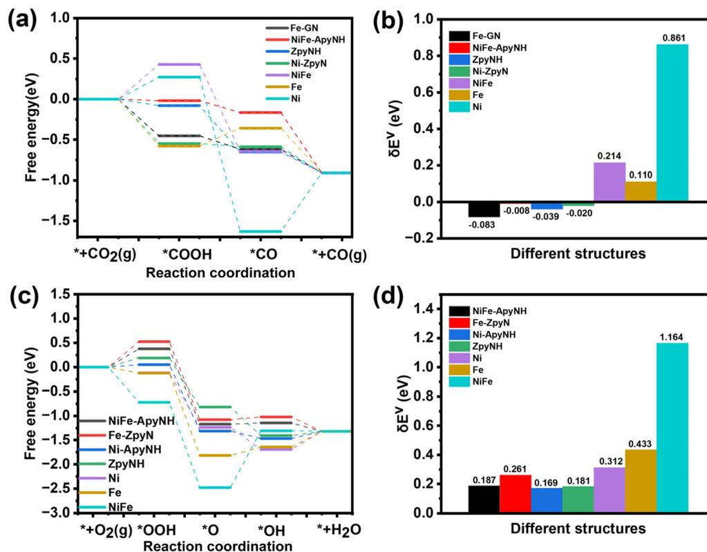
**Fig. 7** The free energy diagrams (FEDs) of CO<sub>2</sub>RR (a) and ORR (c) on optimal active site for each type; (b) the  $\delta E^v$  values of CO<sub>2</sub>RR (b) and ORR (d) on the optimal active site for each type.
