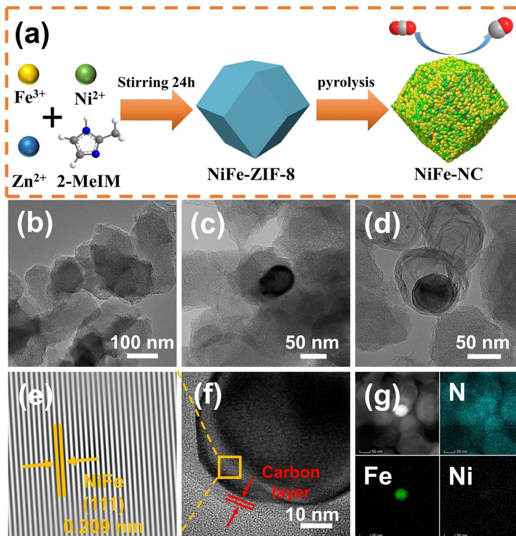
**Fig. 1** (a) Schematic illustration of the synthesis of the electrode material; (b–d) TEM images of NiFe-NC; (e and f) HRTEM images and the magnified image of the selected region for the NiFe alloy nanoparticles; and (g) HAADF-STEM image and EDS elemental mapping images of NiFe-NC.
