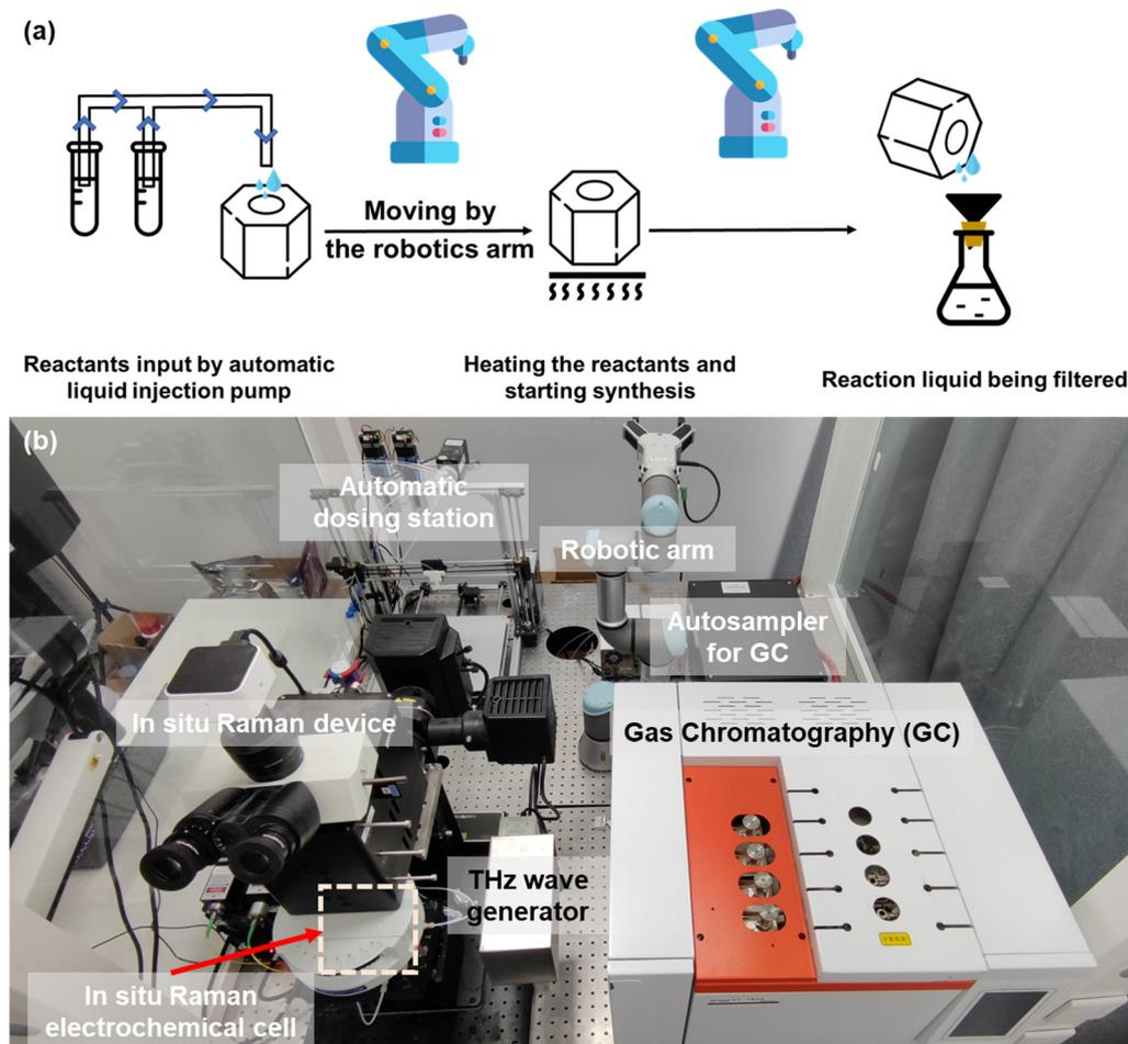
**Fig. 2** (a) Schematic diagram of the robotic-arm-assisted automated MXene synthesis process. Robotic arms moved the heating kettle for safety due to the HF generated during the process. (b) Physical map of the robotic-arm-assisted electrolyte preparation device, electrocatalytic reaction device (*in situ* Raman electrochemical cell), and *in situ* Raman and GC test setup. The THz wave generator was a model CQ-8 THz electromagnetic wave therapy device.<sup>27</sup>
