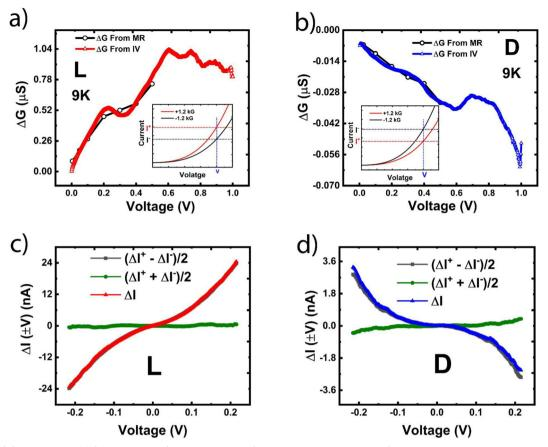
Fig. 5 (a and b) Computation of  $\Delta G$  from I-V data (details in the insets), and comparison with the MC data. A close match has been observed. (c and d) Even and odd parts of the CISS signal  $\Delta I$  in the  $\pm$  0.2 V bias window (non-linear range). The even part is almost negligible, implying that the CISS signal must have an odd functional dependence on the bias.
