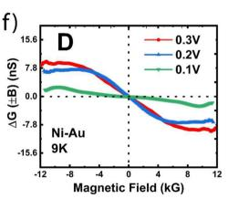
Fig. 4 (a and b) MC measurements on L and D chiral samples, respectively, in the non-linear range ( $\sim 0.5 \text{ V}$  bias). Both forward and backward field scans are recorded. Chirality dependent MC asymmetry is observed, superimposed on a symmetric background positive MC signal. (c and d) Elimination of the background MC signal and  $\Delta G$  vs. B plots. (e and f)  $\Delta G$  vs. B as a function of bias, showing that  $\Delta G$  gradually decreases with lowering bias.
