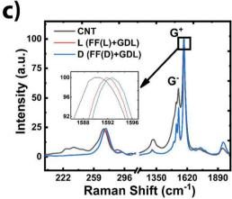
Fig. 1 (a) SEM image of the two-terminal device. Magnetic field B is perpendicular to the plane, and hence perpendicular to all the in-plane (x-y) current paths. (b) CD spectrum of Fmoc-FF (L/D) hydrogels formed in the presence of GdL. (c) Raman spectrum (532 nm laser), showing the characteristic peaks of CNTs before and after functionalization. The inset shows the shift of the G<sup>+</sup> peak due to functionalization.
