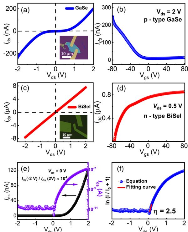
**Fig. 2** (a and c) The output characteristics of individual GaSe and BiSel. The insets show the optical images of the GaSe and BiSel devices. (b and d) The transfer characteristics of the individual GaSe and BiSel. (e and f) The  $I_{ds} \sim V_{ds}$  of the BiSel/GaSe heterojunction and fitting curve.
