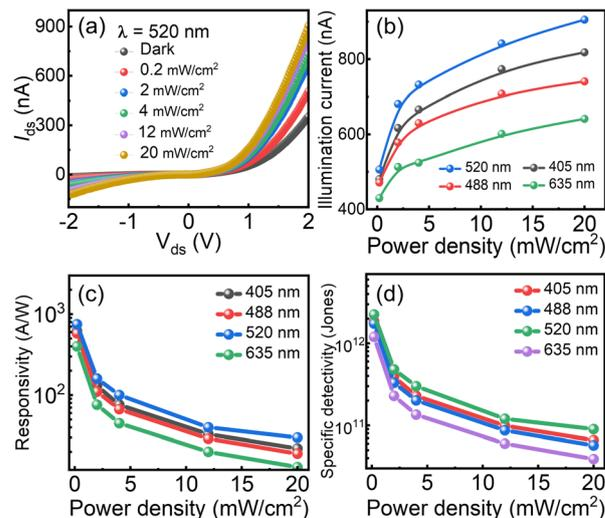
**Fig. 3** (a) The output curve of the device under 520 nm laser illumination with five different power densities of 0.2, 2, 4, 12 and 20 mW cm<sup>-2</sup>. (b) The relationship between power density and illumination current at  $V_{ds} = 2$  V. (c and d) The corresponding  $R$  and  $D^*$  with different power densities at  $V_{ds} = 2$  V under 405 nm, 488 nm, 520 nm and 635 illumination.
