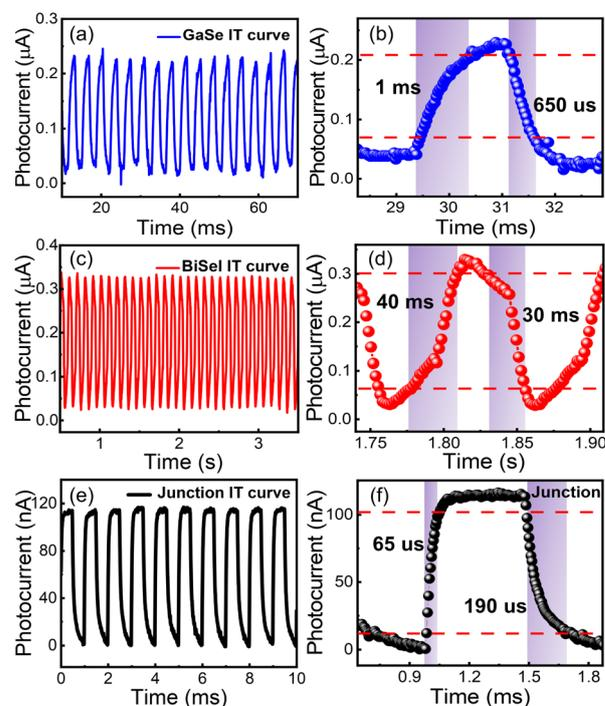
**Fig. 4** The photoresponse to on/off irradiation showing (a, c, and e) the corresponding photodetector stability of GaSe, BiSel and the BiSel/GaSe heterojunction at  $V_{ds} = 2$  V. (b, d, and f) The typical response speed of GaSe, BiSel and BiSel/GaSe heterojunction devices.
