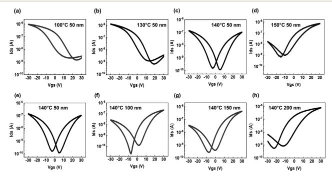
Fig. 2 (a)–(d) Transfer characteristics after 50 nm thickness  $Al_2O_3$  deposition at coating temperatures of 100 °C, 130 °C, 140 °C and 150 °C, respectively. (e)–(h) Transfer characteristics after the  $Al_2O_3$  deposition at 140 °C with coating thicknesses of 50 nm, 100 nm, 150 nm and 200 nm, respectively.
