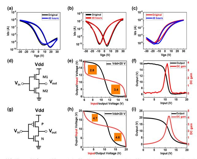
Fig. 4 (a) Stability test of  $Al_2O_3$  coated (a) p-type device, (b) ambipolar device, (c) n-type device. (d) Inverter circuit using two ambipolar devices. (e) Inverter VTC and noise margin at  $V_{dd} = -20$  V and (f) DC gain of the inverter from ambipolar TFTs. (g) Inverter circuit using CMOS device. (h) Inverter VTC and noise margin at  $V_{dd} = -20$  V and (i) DC gain of the inverter from the CMOS device.
